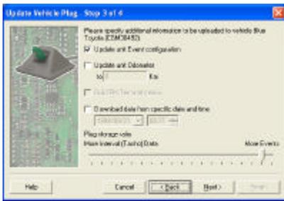
Step 3 shows the options of what can be uploaded to the vehicle. Make sure the Update unit Event configuration is selected. Optionally the Odometer can be updated. The Plug storage ratio determines how much Tachograph data vs. event data is stored in the plug. NOTE: The unit has fixed areas for storing data that cannot be changed. Click next to go to the final step.
